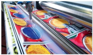
The StarLam 1600R Roll-to-Roll Liquid Laminator applies a smooth, consistent coating of our water-based ClearShield Liquid Coatings, making protecting your digital prints a quick & simple process. The StarLam handles of a variety of substrates up to 64" wide, and with our various ClearShield formulations, you will find the perfect coating solution for your application. Our innovative and proven system offers a cost effective laminating solution.
