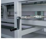
Linear guided height adjustment by means of hand wheel
