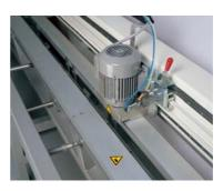
• Pneumatic blade clamping
